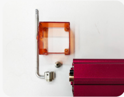
Remove the protective cover, air guide cover, nozzle, and window mirror.
